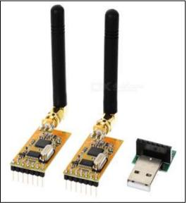
Fig. 4: RF transmitter and Receiver module
