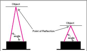
Fig. 3: IR sensor triangulation principle
