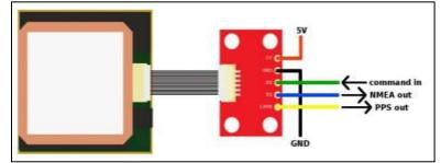
Fig. 2: EM406 GPS with EM406 Breakout
